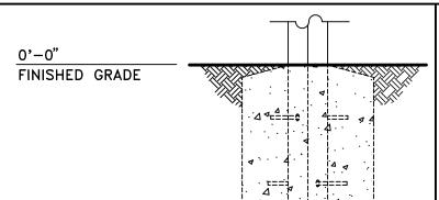
NOTE: CONCRETE AND NO. 4 REBAR BY OTHERS
