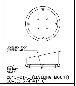
TIMBERFORM RENAISSANCE MODEL NO. 2815-DT LITTER CONTAINER, SIDE EMPTY WITH DOME TOP
